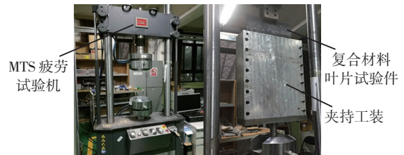
图3 复合材料风扇叶片拉伸试验夹持及加载系统 Fig.3 Clamping and loading system of tensile experiment on the composite fan blade
